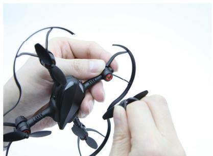
b. Attaching a propeller
