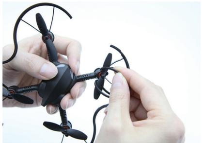
Then firmly pull upward from the center to remove the propeller.
