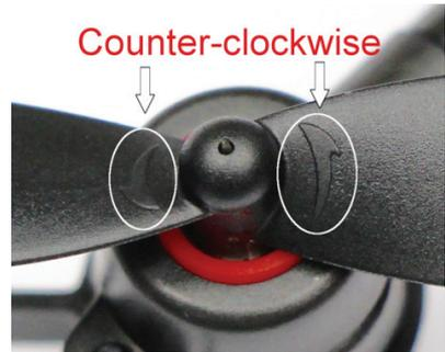
iii. For proper lift, the propellers need to be arranged as shown below.
