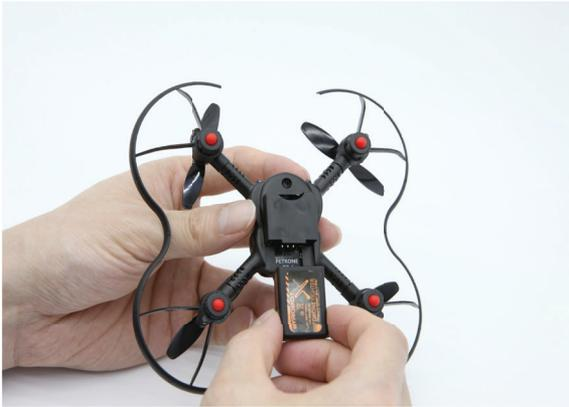
When the battery is fully inserted into the Petrone, the LED lights will light up.
