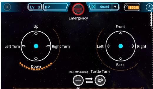
The left joystick handles vertical controls (moving up and down) and orientation (turning left and right).
